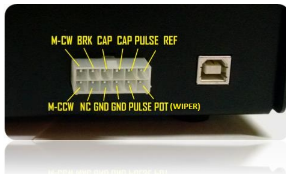
Figure 13: Board scheme for YAESU G450/G650
